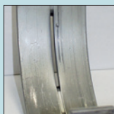
Grooving through abrasion (Bearing ring)
