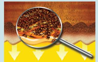
*The CJC™ Fine Filter Insert purifying the oil until the cellulose fibres are completely saturated.*
