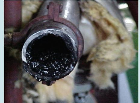
***Oil degradation products are the major cause of these problems which can be avoided with a continuous fine filtration of the thermal oil.***
