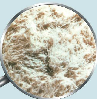
Because of their structure CJC™ Fine Filter inserts are comparable with a labyrinth-like, extremely close-meshed volume sieve with finest, countless branched channels. The total volume of cavities of the filter insert amounts to 75% which explains the particularly high dirt holding capacity.
