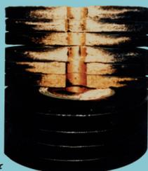
*Sectional view of a used CJC™ Depth Filter insert*
