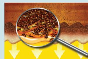
*The CJC™ Fine Filter Insert purifying the oil until the cellulose fibres are completely saturated.*
