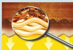
*Oil degradation products deposit at the cellulose fibres (combination of adsorption and absorption)*
