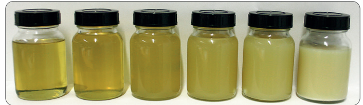
Hydraulic oil samples with various water content.
