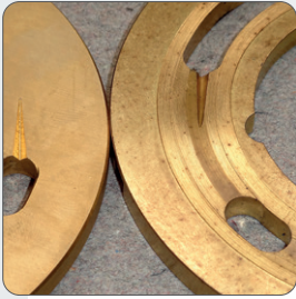
Grooving through abrasion (pump)
