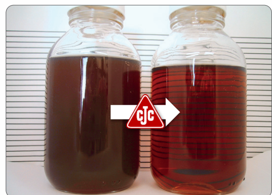
Oil samples left: zero sample, right: with CJC® Cooling Lubricant Filter
